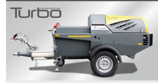
The new SP 20 THF is a worm pump for self-levelling floor screed applications. Equipped with a 4 cyl. turbocharged Kubota diesel engine with 33 kW, this machine is more powerful and allows high delivery distances.
